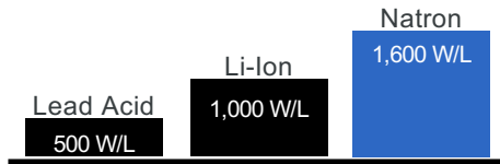
Discharge Power Density
